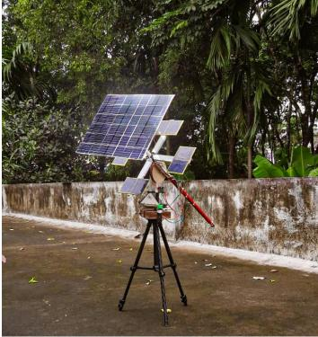
This figure shows the working model of the solar tracker system. The whole system is light-weight as panel casing is removed and structure is made of aluminium. With proper casing and wiring the whole system can be made waterproof. Thus, ensuring the functioning of the entire project during any season.
