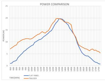
The Power output of both flat panel and solar tracker was calculated with the help of a Power Logger. This was done with the help of Arduino and INA219 IC which was used to calculate both Voltage and Current. By multiplying both these values power was calculated. This power was logged in the interval to 10 minutes. After doing these reading simultaneously, following results were obtained:
