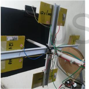
The figure represents the Tracker system controller. It makes the system move by powering motor by small panels. Thus, it makes the arrangement super simple and both the x and y axis can be controlled by it.
